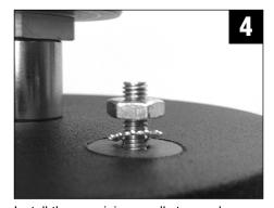
Install the remaining small star washer over the projecting screw and secure with the nut.
