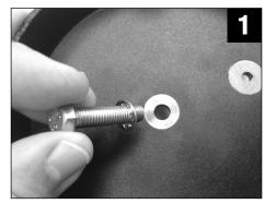
Place the large star washer on the bolt and, from the underside, run through the center hole of the base.
