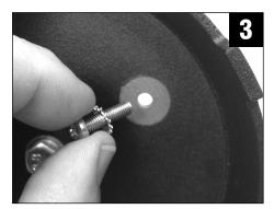
Place a small star washer over the Phillipshead screw and, from the underside, insert through the remaining hole in the base.
