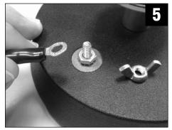
Attach the cable to the projecting screw using the wing nut. Notice the orientation of the lug - this eases the tightening of the wing nut.
