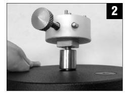
Place the bushing over the projecting bolt and screw on the vise. Use the wrench to tighten the bolt.
